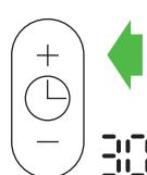
To set the sleep timer, select the desired time. When time reaches zero, the appliance will go into standby mode. To cancel, reduce the time until two dashes appear.
