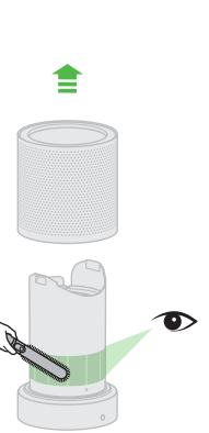
Look for blockages in the small aperture inside the loop amplifier. Use a soft brush to remove debris.
