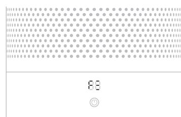
When your non-washable filter unit needs replacing the appliance will display the pattern shown. To replace the non-washable filter unit, follow these steps.
