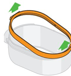
Unclip the loop amplifier surround: pull from both sides of the lower tab, gently but firmly.
