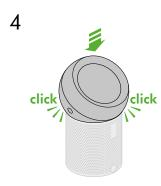
Firmly push the ball back into position, making sure it clicks securely into place.
