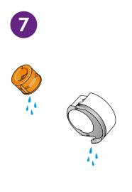
Unclip the cap, take the evaporator out of the water tank and rinse under a cold tap.
