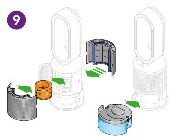
Push the evaporator back into your machine, making sure that it is securely in position.
