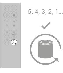
Important: Reset your filter level Press and hold the Night mode button on the remote control.
