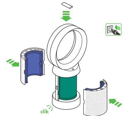
Position the shrouds onto the base and push gently until they click securely into place.
